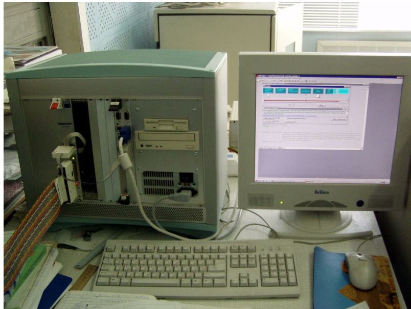
Figure 1. The prototype of Altera FPGA-based scalable correlator PARSEC with Mark IV specification.
