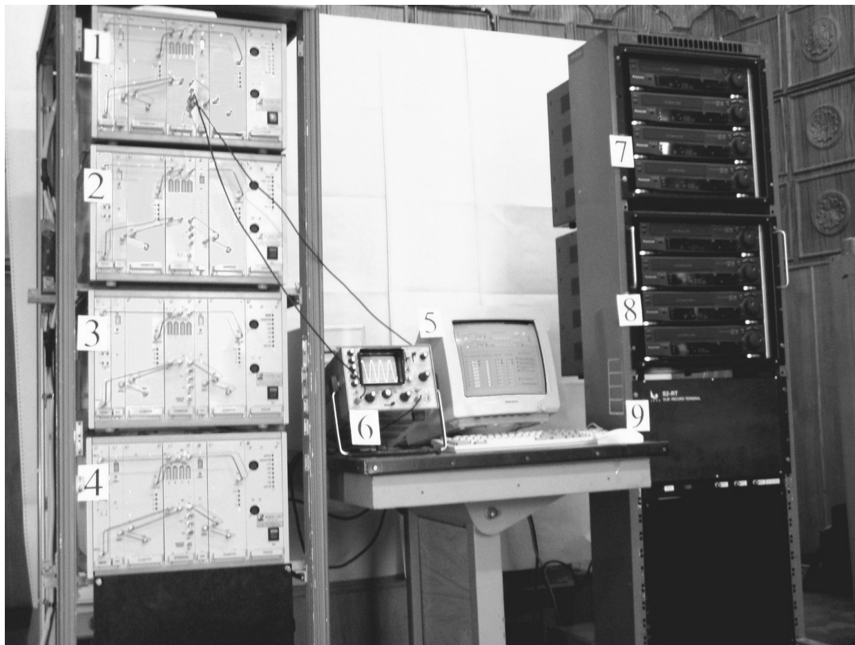
Figure 4. 8-channel DAS with S2-Rt recoding terminal: 1, 2, 3, 4 — DAS modules; 5 — control PC; 6 — oscilloscope for phase calibration signal monitoring; 7, 8, 9 — S2-RT modules.
