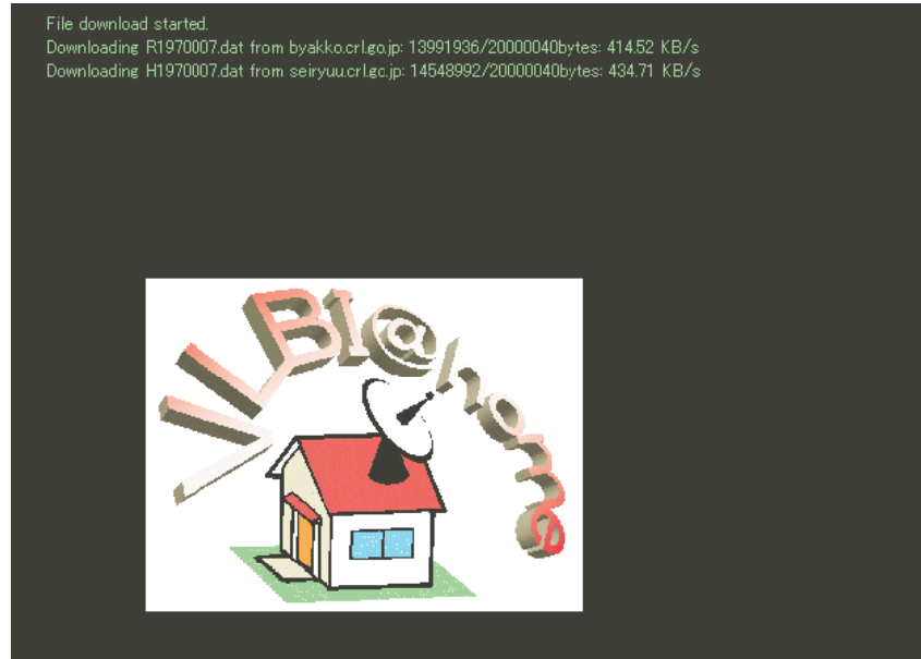
Figure 3. Screenshot of screensaver-type client program downloading two VLBI raw data simultaneously. Two data are cross-correlated by a XF-type software correlator and result data are sent back to a server.
