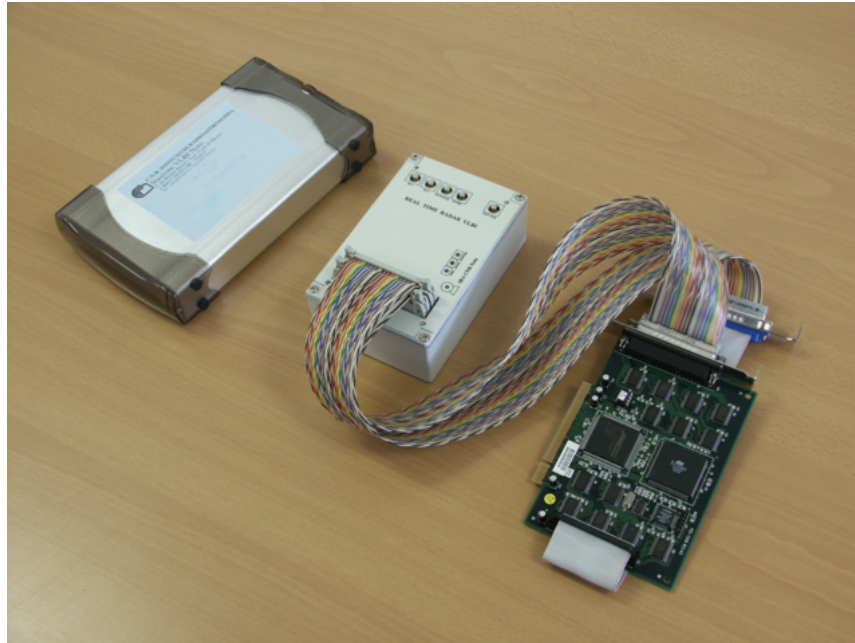
Figure 1. The entire acquisition terminal is shown: from the left side, an external Firewire/USB2 disk, NRTV Box, a commercial PCI board.
