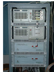
Figure 2. CVN harddisk system playback unit (upper) with playback interface (lower).
