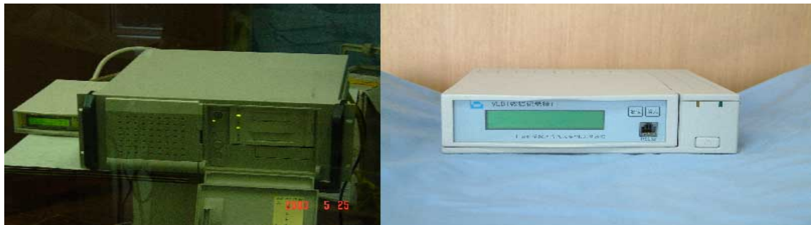
Figure 3. CVN harddisk system (left) with the record interface.
