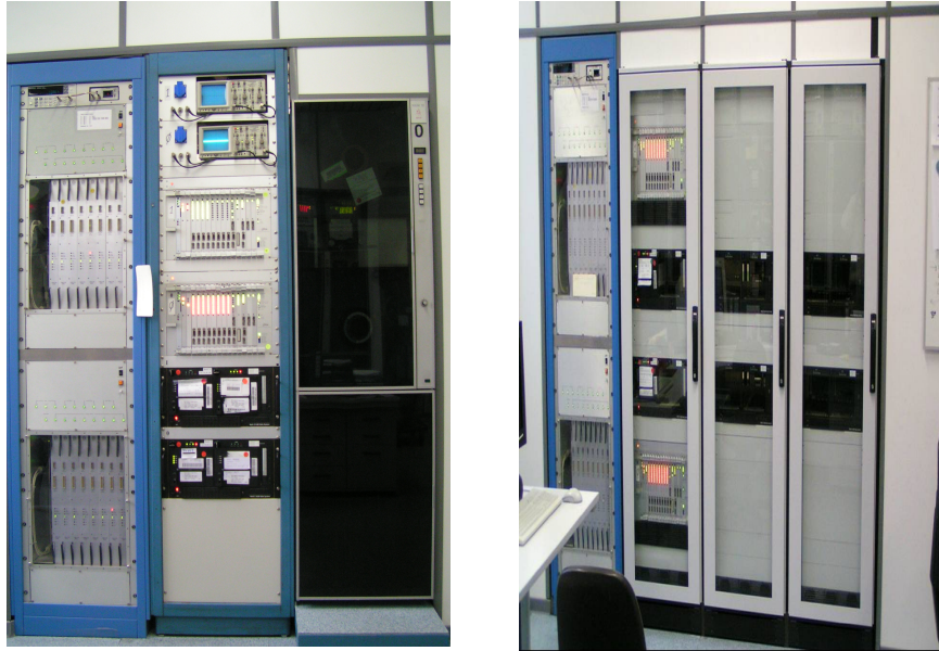
Figure 1. Left: Part of the MarkIV data processor: correlator rack with two Mark 5 playback units and two station units as well as one playback tape drive. Right: one of the three new racks equipped with three Mark 5B units and space for the correlator interface boards (CIB).
