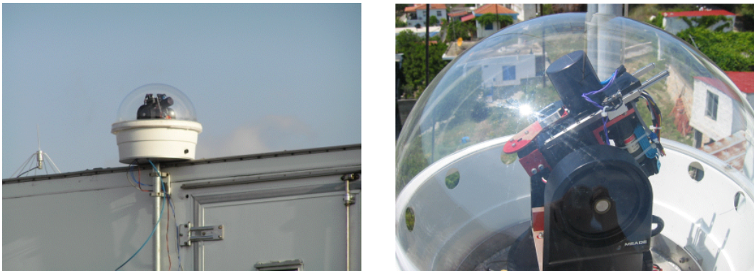
Figure 2. Solar Spectrometer GEMOSS from ETH-Zürich.
