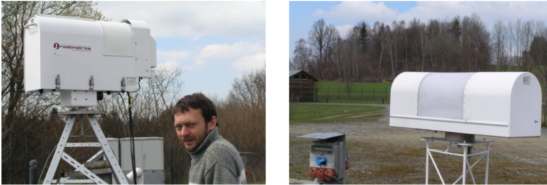
Figure 1. Water Vapour Radiometer built (a) by Radiometrics and (b) by ETH-Zürich.
