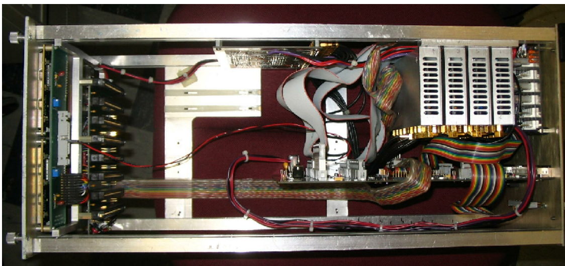
Figure 3. Photograph of a Mark IV Formatter converted to a Mark 5B Sampler Module
