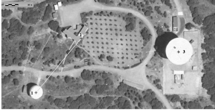
Figure 1. The IGN facilities at Yebes (Guadalajara, Spain). Displayed are (1) the 14-m radiotelescope used in VLBI observations, (2) the GPS antenna of the IGS station, and (3) the new 40-m radiotelescope
