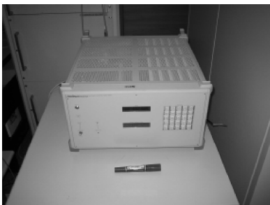
Figure 4. LD-pumped cesium gas-cell atomic frequency standard
