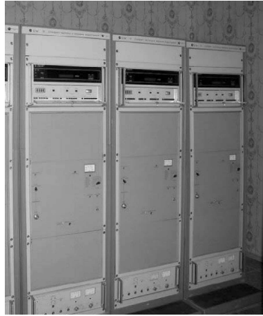
Figure 1. The set of active hydrogen standards CH1-80, observatory “Zelenchuk-skaya”
