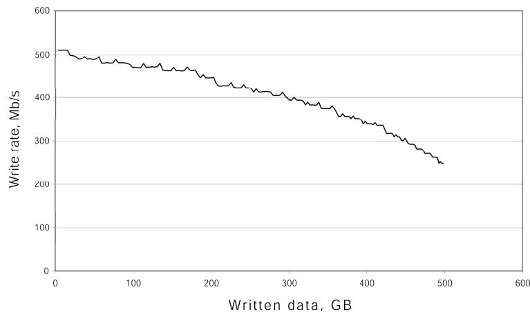
Figure 1. Single Hitachi 500 GB disk drive
