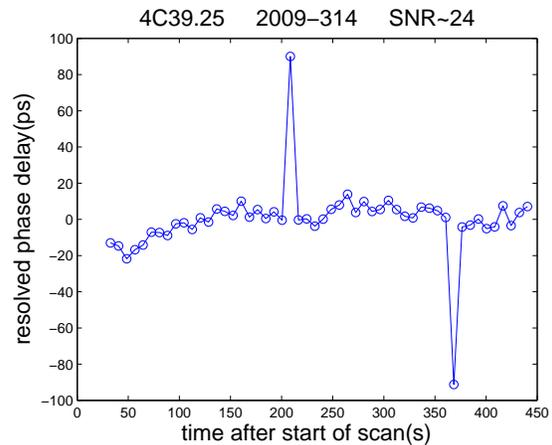
Figure 4. Phase delays for a 450-s scan of 4C39.25 taken on day 314 of 2009. The scan is divided into 8-s segments, each with an SNR of about 24. Cycles of phase were resolved independently for each segment using the bbd technique.
