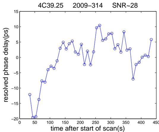
Figure 3. Phase delays for a 450-s scan of 4C39.25 taken on day 314 of 2009. The scan is divided into 10-s segments, each with an SNR of about 28. Cycles of phase were resolved independently for each segment using the bbd technique.
