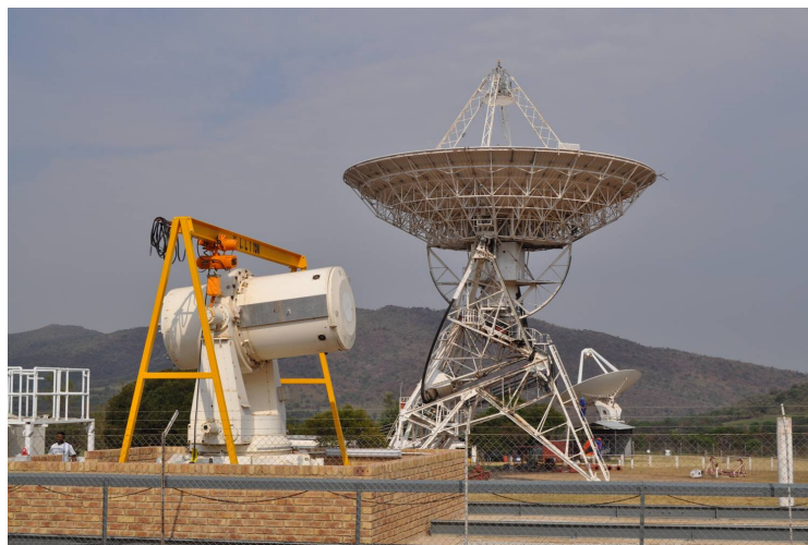
Figure 1. 1-m Cassegrain (ex OCA) which will be used as part of an SLR/LLR system being developed at HartRAO, with the 26-m VLBI antenna (mid-background) and the 15-m SKA prototype (far background). The 15-m antenna is being equipped for S/X VLBI and will be used for IVS EOP measurements.
