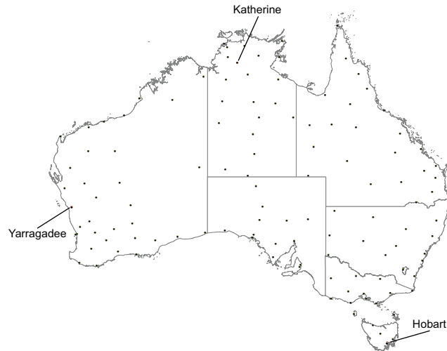
Figure 1. The geographical distribution of VLBI and GNSS infrastructure for AuScope. The locations of the new 12-m telescopes are labelled, and the new GNSS sites are indicated by filled dots.
