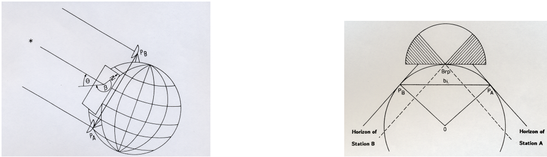
Figure 1. Left: example of the midpoint based reference system (notice that this picture presents a baseline used in polar motion measurements, for dUT1 measurements a East-West placed baseline is needed). Right: geometry of baseline reference system and horizon mask are shown (pictures from [1]).
