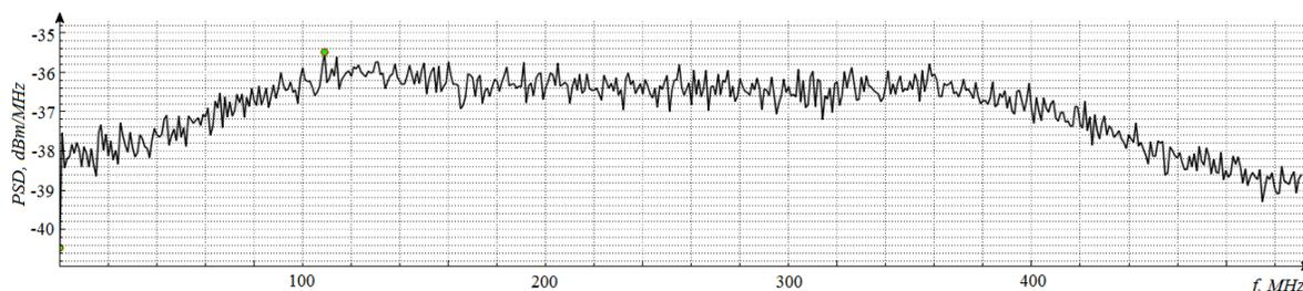
Fig. 5 PSD estimated by using captured input signal in X-band at the Zelenchukskaya observatory.
