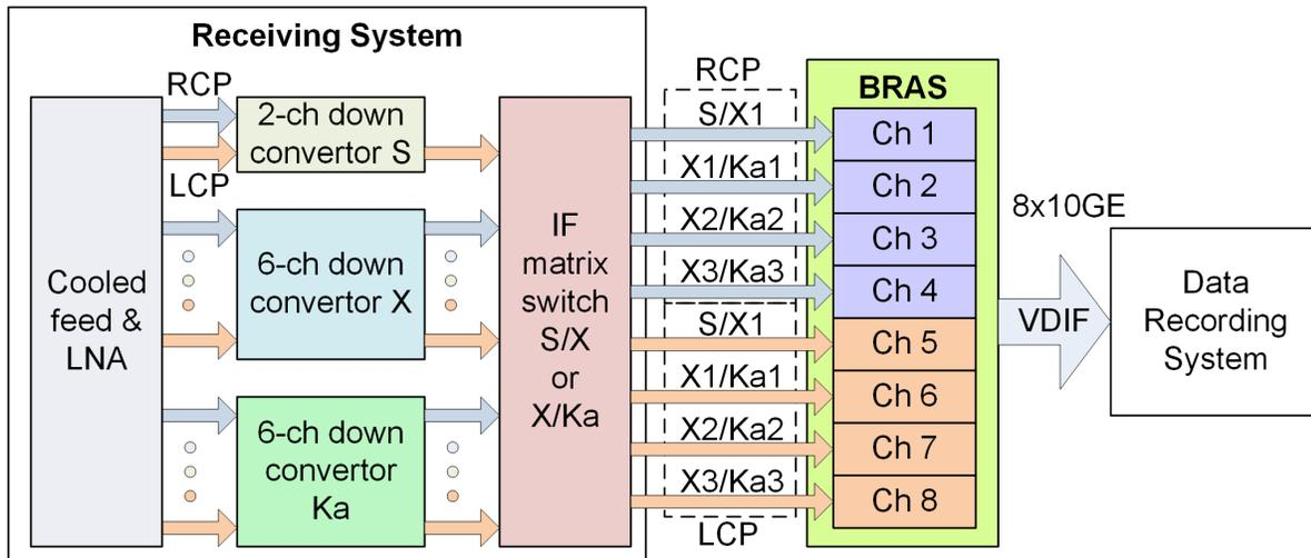
Fig. 2 Signal chain of the RT-13 radio telescopes.
