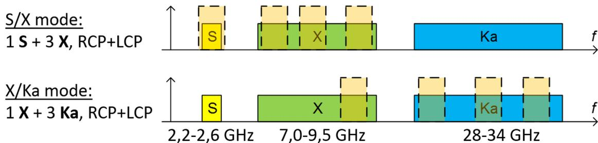
Fig. 3 Switching modes of the RT-13 radio telescopes.
