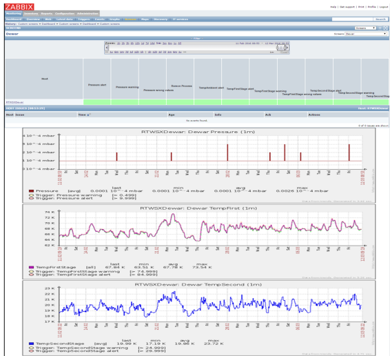
Fig. 3 A possible Web page showing the monitoring data which are collected from the cryo-system of the dewar.
