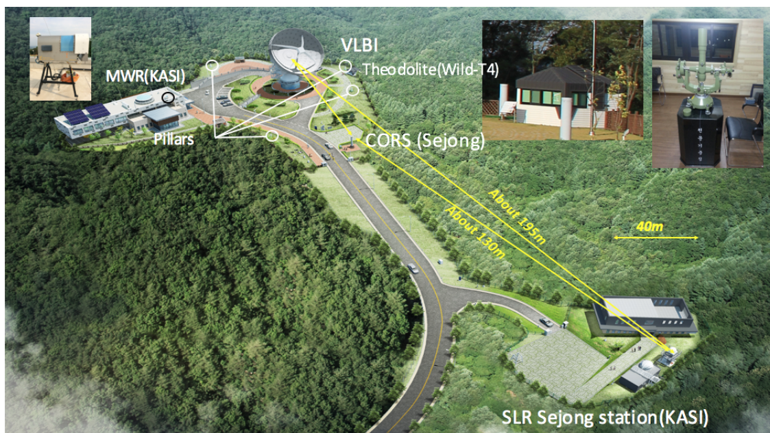
Fig. 1 Site layout and equipment at the Sejong station (KASI's newly installed SLR station in October 2015).
