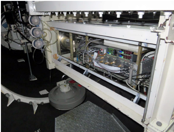
Fig. 2 New S-/X-band VLBI receiver at O'Higgins.
