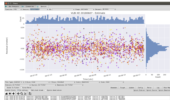
Fig. 2 The There graphical analysis tool. The plot shows post-fit residuals (after the Estimate stage) for the XE session on June 7, 2018. The colors indicate the baseline. That is, all residuals for the same baseline have the same color.
