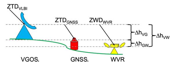
**Fig. 4** Sketch showing a co-location site with three different instruments and the heights of their respective reference points. In order to meaningfully compare atmospheric parameters, corresponding height corrections need to be applied.
