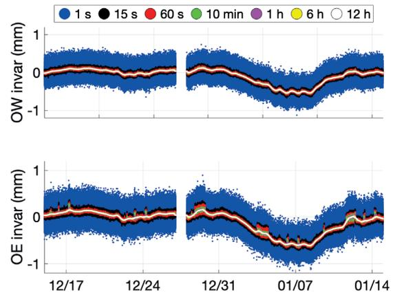
**Fig. 2** The first month of measurements with the new OTT invar systems. Shown are the original data with a temporal resolution of 1 s (blue), as well as moving averages with bin sizes of 15 s (black), 60 s (red), 10 min (green), 1 h (magenta), 6 h (yellow), and 12 h (white).
