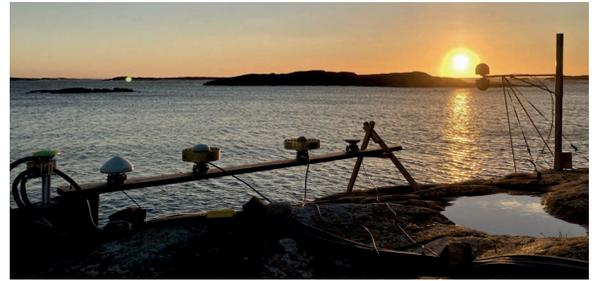
**Fig. 7** GNSS antennas used for sea level monitoring.
