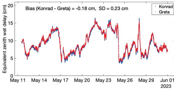
**Fig. 5** Two-minute averages of the equivalent ZWD inferred from observations with Greta (red dots) and Konrad (blue dots).
