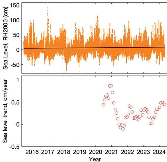
**Fig. 6** Top: hourly mean values of the sea level from the tide gauge station at OSO in the Swedish observational network. Bottom: the linear sea level trend estimated up to a specific time on the X axis starting from 2020.
