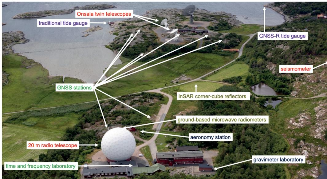
**Fig. 1** Aerial photo of the Onsala Space Observatory depicting the location of the telescopes and other geoscientific instrumentation.
