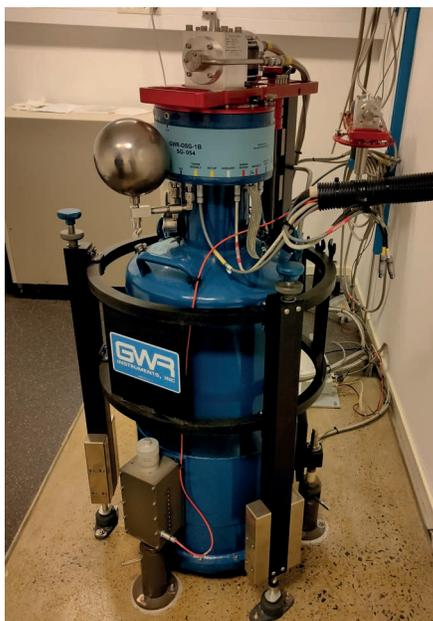
**Fig. 4** The superconducting gravimeter SG054.
