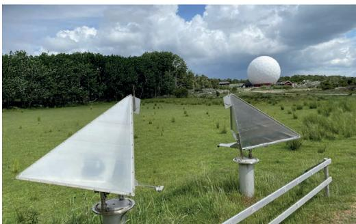
**Fig. 9** The InSAR reflectors at OSO.
