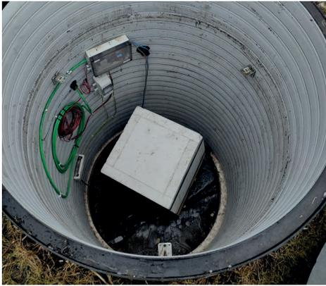
**Fig. 8** The seismometer is installed on solid rock at the bottom of a 2 m deep well. It is covered with cellular plastic, and the well is surrounded by soil to reduce rapid temperature variations.
