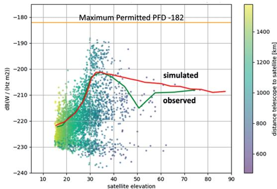
**Fig. 3** Power Flux Density versus Elevation: Simulated vs. Observed. Note that at  $El > 35^\circ$  the data are sparse as there are few satellites at high elevation, and the LEO sat beams are better defined and the projected beam spillover is less.
