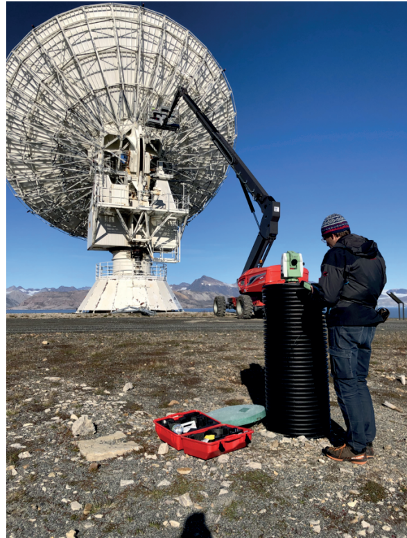
Fig. 8 Halfdan Pascal Kierulf during the last local-tie measurement campaign with the 20-m antenna (Ny) in the background before the decommissioning.
