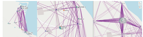
Fig. 3 Observation lines between the old and new observatories (left), around the new observatory (middle), and towards rotating reflectors on the VLBI dish.
