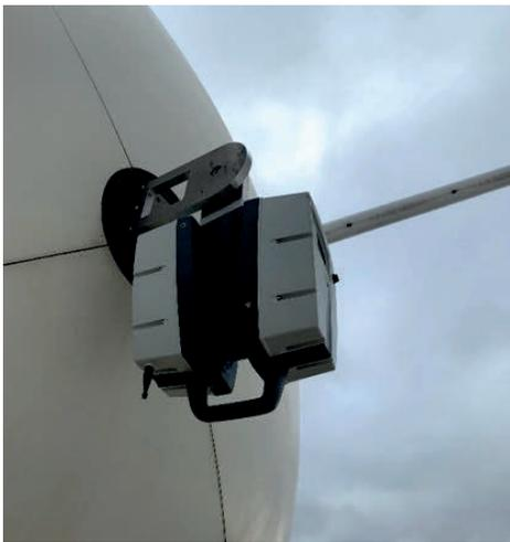
Fig. 2: Leica ScanStation P40/P30 laser scanner.
