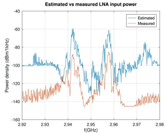
Fig. 6 Estimated and measured total power at LNA input.
