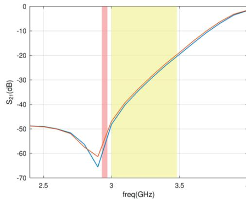
Fig. 3 Measurement of S21 COTS filters.
