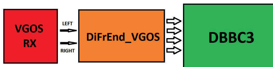
Fig. 1 Schematic view of the DiFrEndVGOS in the DBBC3 environment. No filters are required to select the input bands in the DBBC3. Those are digitally generated by the DiFrEnd module and so are flexibly selectable in the VGOS band.
