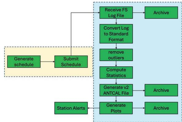
**Fig. 1** Flow chart for processing antenna telemetry from FS logs. The shaded blocks indicate processes that are automated, with the yellow shade representing only the single-dish experiment (SDE) automation and blue indicating automation for all logs.
