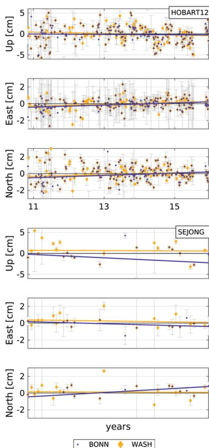
**Fig. 5** Station position residuals for HOBART12 and SEJONG. The solid lines describe a linear fit.
