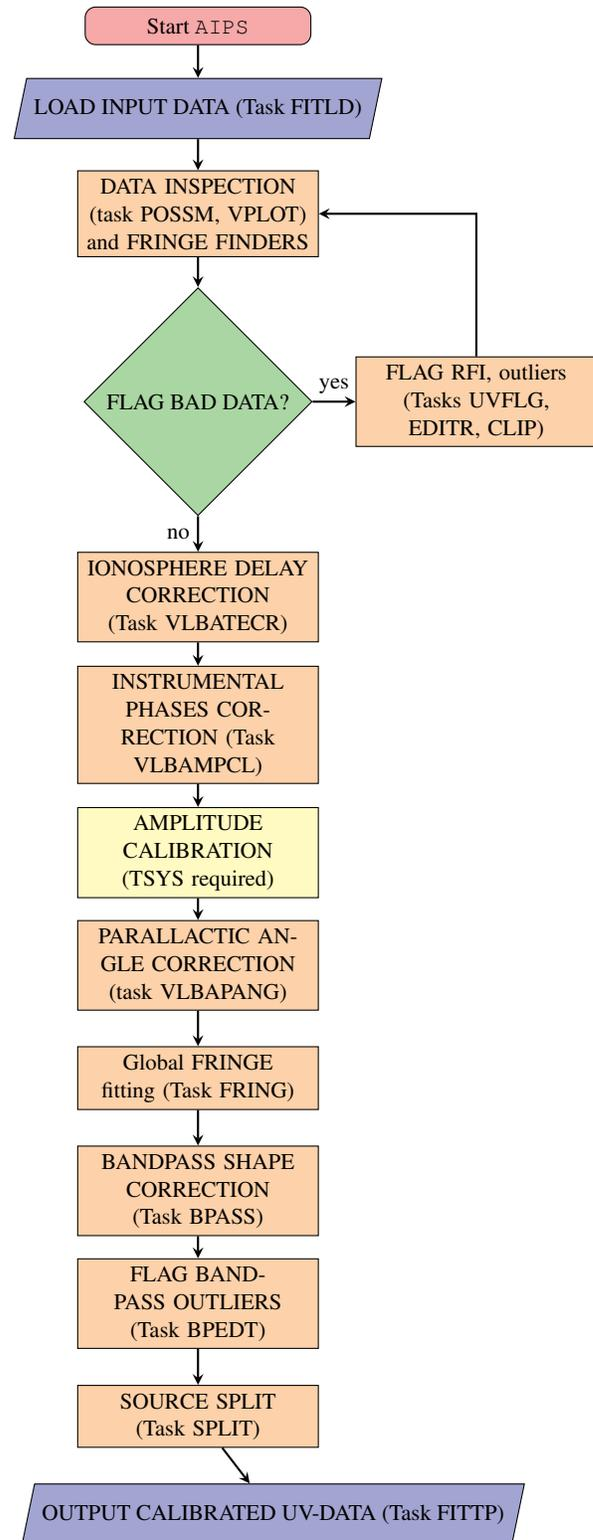
**Fig. 1** Flowchart of the current calibration pipeline of VGOS data in AIPS. This does not include amplitude calibration for session VR2201, as no TSYS information is available.
