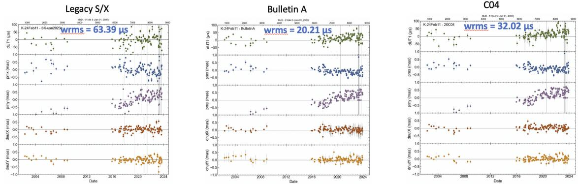
**Fig. 2** EOP residuals of 24-hour K-band diurnal sessions compared to S/X data from usn2023c global solution, Bulletin A, and IERS C04.
