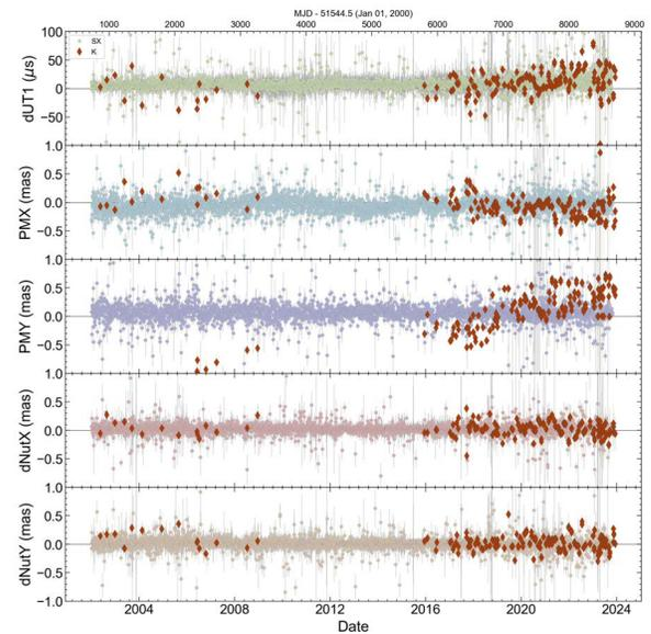
**Fig. 3** EOP residuals for the K-band 24-hour diurnal sessions compared to the legacy S/X band data from the C04 series.
