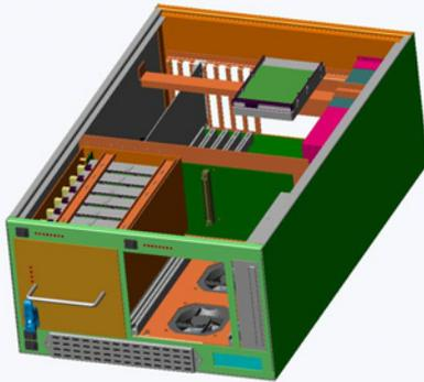
*The new Mark 5 chassis design drawing shows one 8-pack module installed in the left front of the chassis. The right front is empty, ready for a second 8-pack module to be inserted.*
